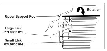
Figure 11. Removing Conveyor Belt Chain
