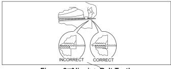
Figure 9. Aligning Belt Teeth
