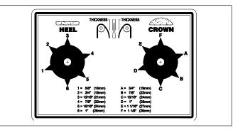
Figure 4. Bun Thickness Adjustment Controls
