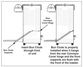
Figure 1. Installing Bun Chute
