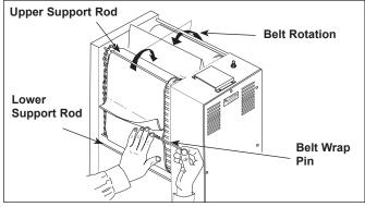
Figure 8. Installing Belt Wrap
