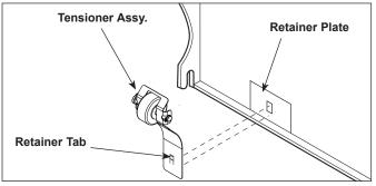
Figure 13. Replacing Roller Tensioner Assy.
