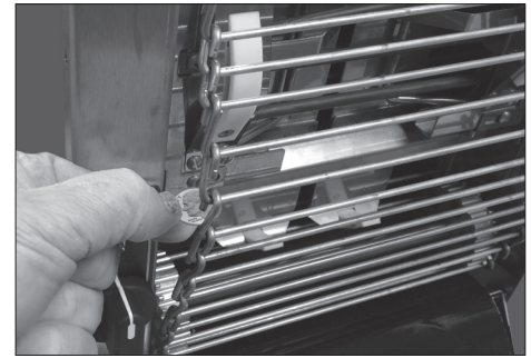
Figure 10. Measuring Conveyor Belt Chain
