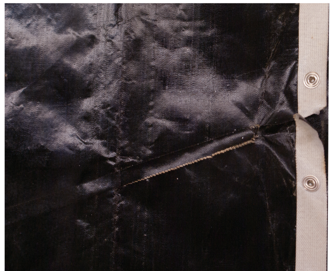
ABOVE: Belt is torn and missing a snap. Replace belt.
