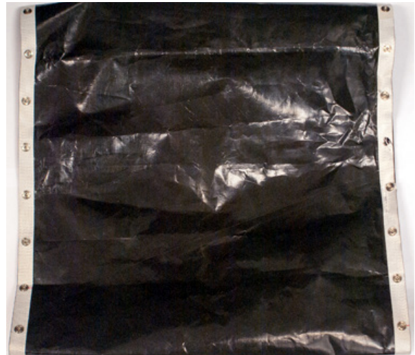
ABOVE: Belt is folded. Edge of belt on right is torn and missing a snap. Replace belt.
