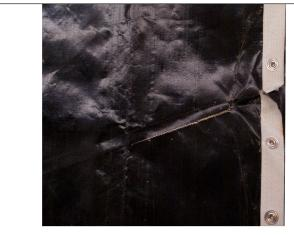
**BELT IS MISSING SNAPS** AND IS DAMAGED. REPLACE BELT. Figure 6. Example of Damaged Belt
