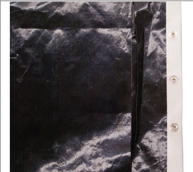
BELT IS TORN AND FOLDED. REPLACE BELT.
