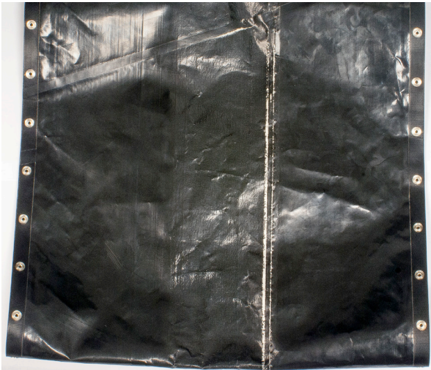
ABOVE: Belt is folded and shows a worn crease down the middle. Replace belt.
