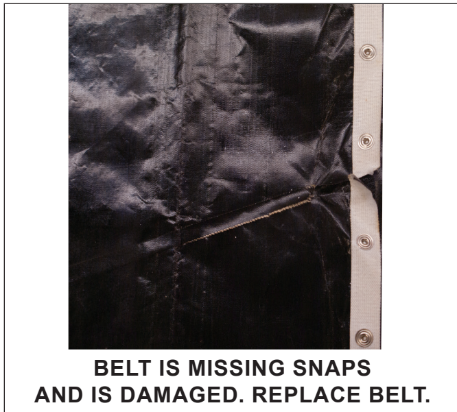
Figure 6. Example of Damaged Belt
