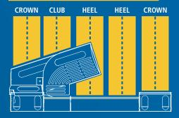
The HEBT-5V has five toasting lanes—two for crowns, two for heels, and one for clubs—and a dual bun feeder that provides access to both sides of the prep line, which allows the toaster to be seamlessly integrated into every McDonald's operation.
