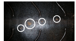
Failed Belt Wrap - Worn.
