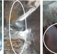
Failed Release Sheet Butter burnt/caramelized on release sheet.
