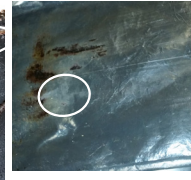
Failed Release Sheet (White Spot) from excessive scrubbing.
