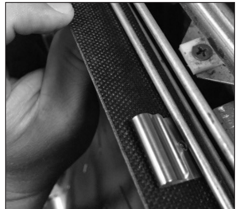
Figure 6. Connect Belt Wrap Hooks
