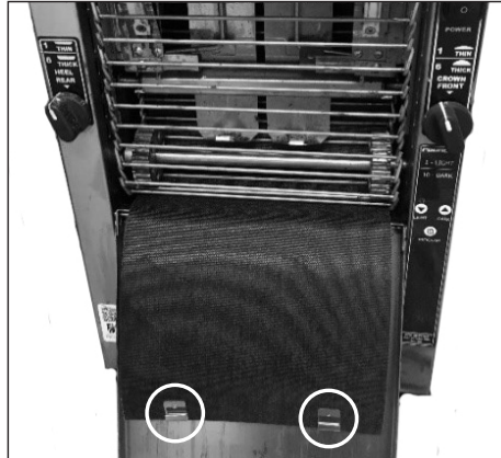
Figure 5. Replacing Belt Wraps
