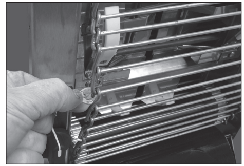
Figure 9. Measuring Conveyor Belt Chain
