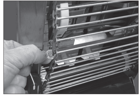
Figure 9. Measuring Conveyor Belt Chain
