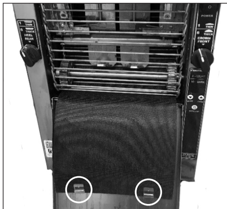
Figure 5. Replacing Belt Wraps
