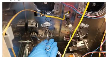
Reinstall both bearings and both retainers. Secure with hex nuts. DO NOT over tighten hex nuts.
