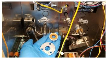
Install two (2) washers onto each of the two (2) drive shafts.Ensure the washers are pushed all the way onto the drive shafts.
