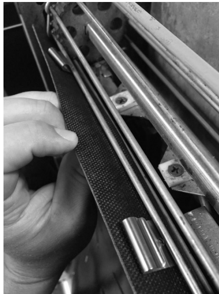
Figure 16. Remove Belt Wrap Hooks
