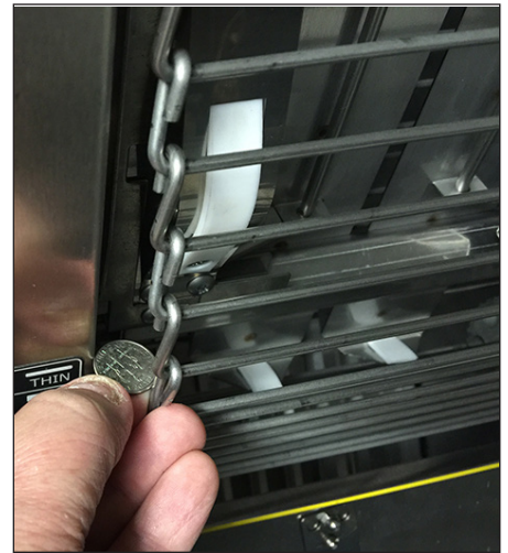
Figure 17. Measure Conveyor Belt Tension
