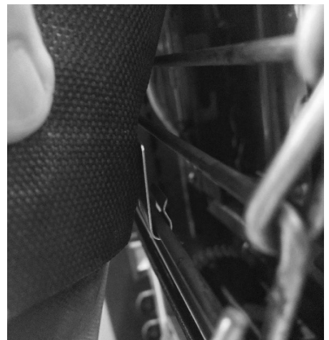
Figure 19. Connect Belt Wrap Hooks
