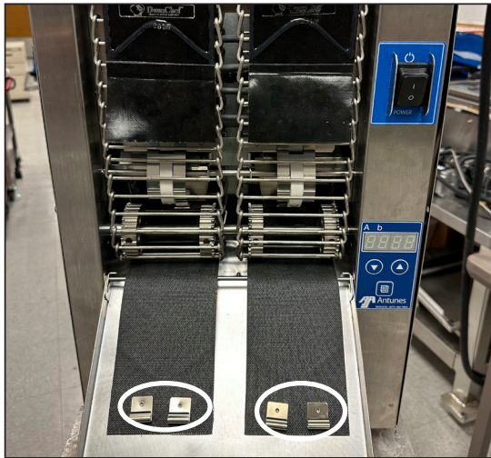
Figure 6. Replacing Belt Wraps
